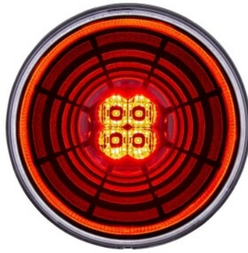
Item No. 36566 13 LED 4" Round Abyss Light (Stop, Turn & Tail) - Red LED/Clear Lens
